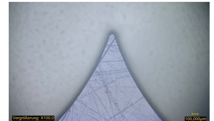
Shape free cutting of a ceramic
