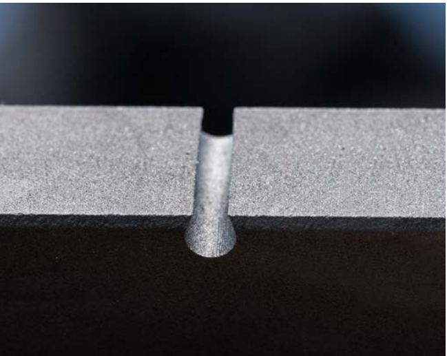
Side view of a laser cut (SiC, material thickness 8 mm)
