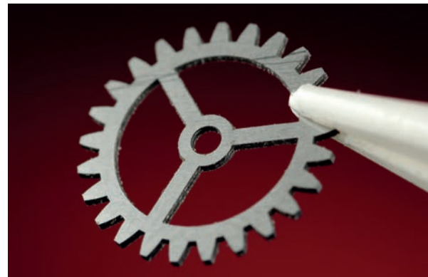
Demo part with burr-free precision cuts
