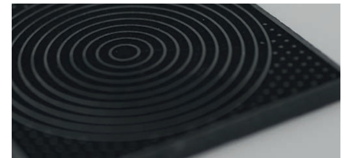
As an ablative procedure, the material areas around the pins to be produced are specifically removed
