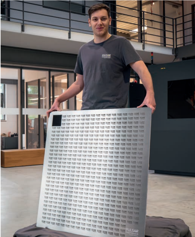
Demonstrator plate (1000 mm x 1000 mm) for large-area USP laser processing with sample structures for functional surfaces and deep engraving.
