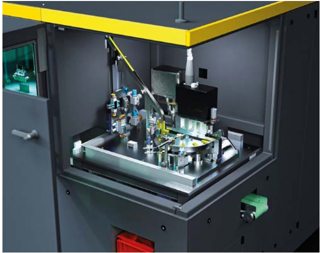
Interior of the P1000 automatic with rotary indexing table and several machining, handling and measuring stations
