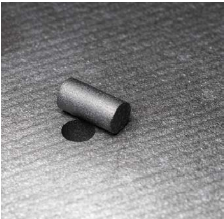
Deep hole drilling in technical ceramics (SiSiC, material thickness 10 mm)
