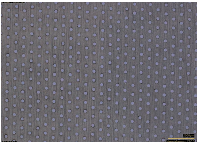
Microscope image: Result of a QCW drilling process in stainless steel
