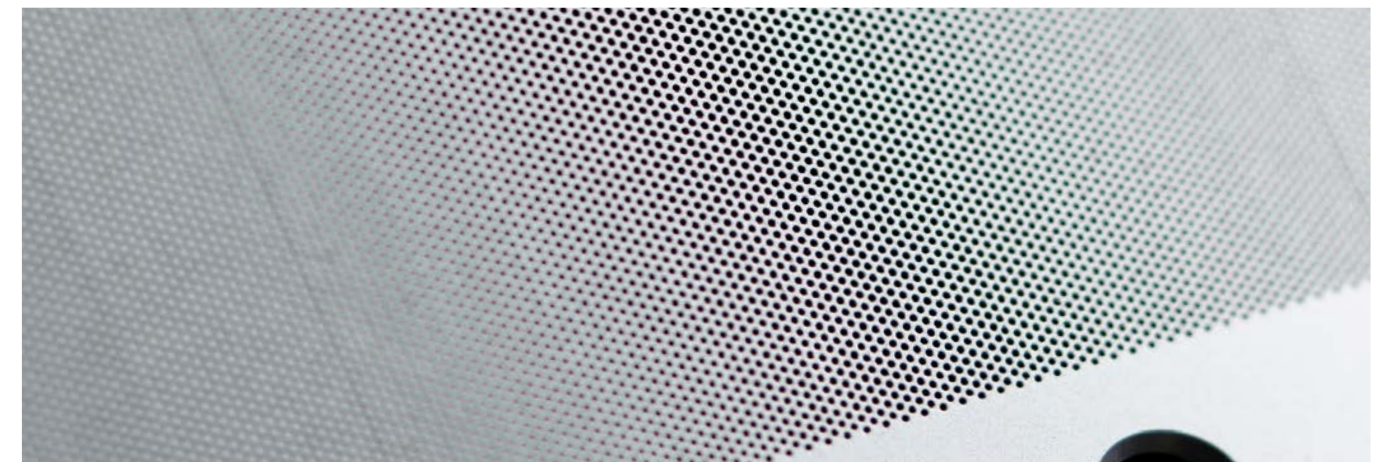
QCW holes of a sieve (after cleaning step)
