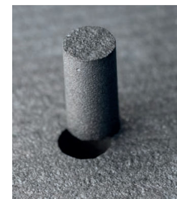
Deep hole drilling in technical ceramics (SiSiC, material thickness 10 mm)
