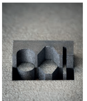
Free-form contour cut in 3D-printed SiC-ceramics, material thickness 5 mm.
