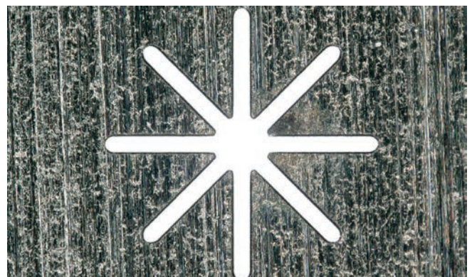
Star-shaped microcuts in stainless steel
