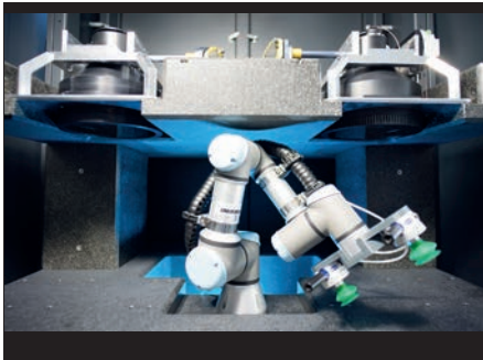
Robot-assisted component feeding in a dual-head setup as a configuration example
