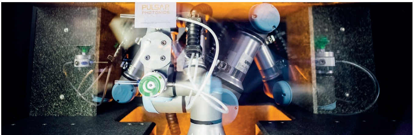
Customized system with automatic workpiece magazines and an integrated UR robot
