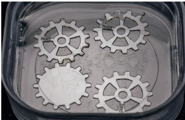
UKP laser cutting parts
